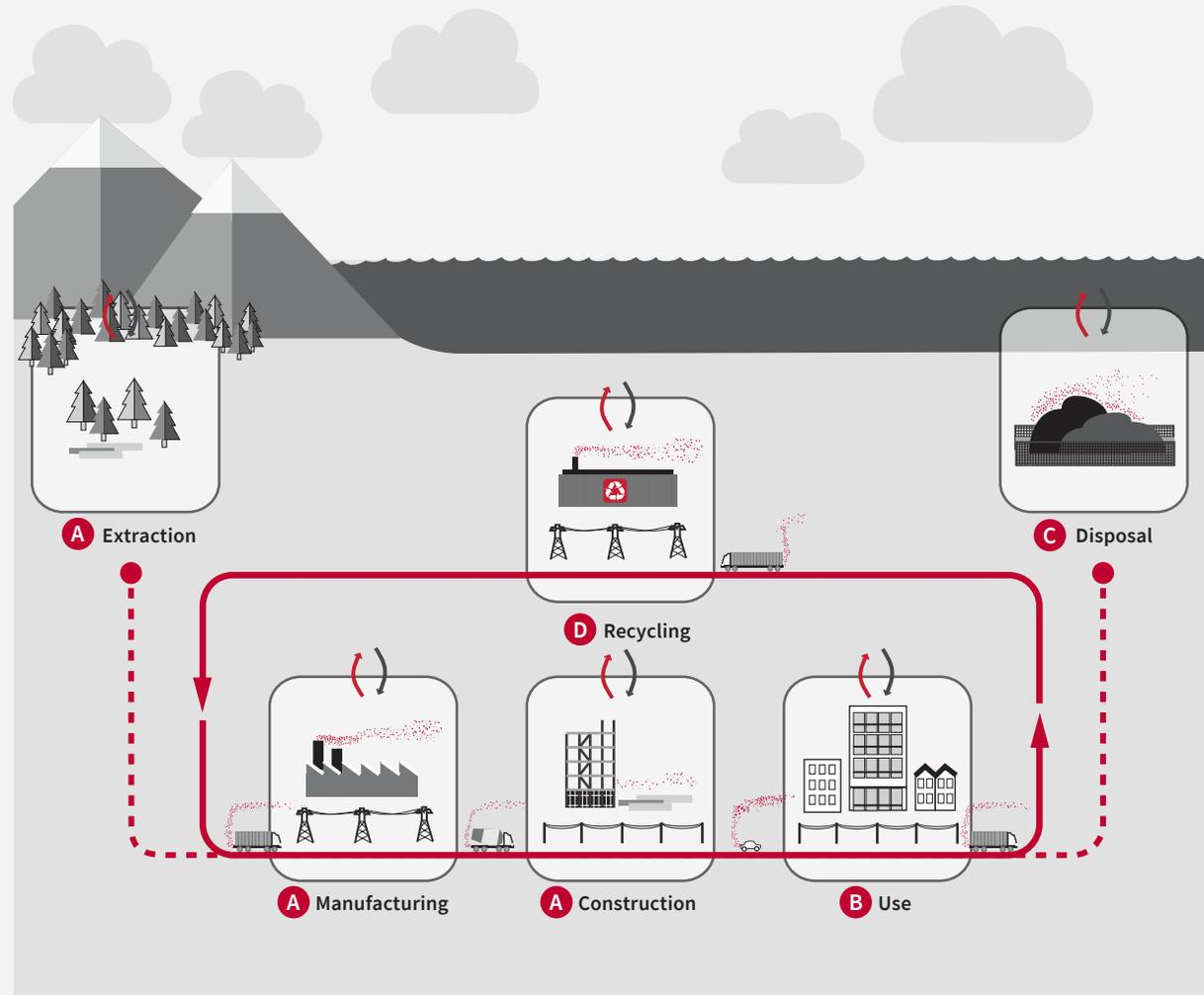
**Figure 1.** Sources of emissions by life cycle stage (A, B, C, D) of a building based on stage definitions from European Standard (EN) 15978 (credit: Meghan Lewis).
